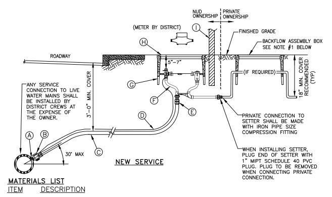
(A) DIRECT TAP: DIRECT TAP OF DUCTILE IRON OR CAST IRON LARGER THAN 4" DIAMETER IS REQUIRED FOR 1" SERVICES. SADDLES WILL NOT BE ALLOWED ON DUCTILE IRON OR CAST IRON PIPE LARGER THAN 4" DIAMETER.
