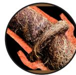
**TREE ROOT INFILTRATION.** This occurs more frequently with older pipes. Modern side sewer pipes are heavy-duty, water-tight plastic which last much longer.
