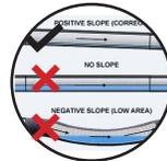
**GRADE/SLOPE PROBLEMS.** If the slope of your private sewer line is too gradual or flat, you may encounter more frequent blockages. (Photo courtesy of [www.hydro-physics.com/common-problems/](http://www.hydro-physics.com/common-problems/))
