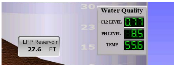
A remote monitoring system reports water quality data at NUD's Lake Forest Park storage reservoir.
